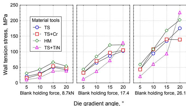
Fig.9 - Change of wall tension stress independence on die gradient angle and blank holding force for various tool materials
