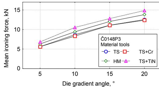
Fig.3 - Change of mean value of drawing force in dependence on die gradient angle for various tool materials
