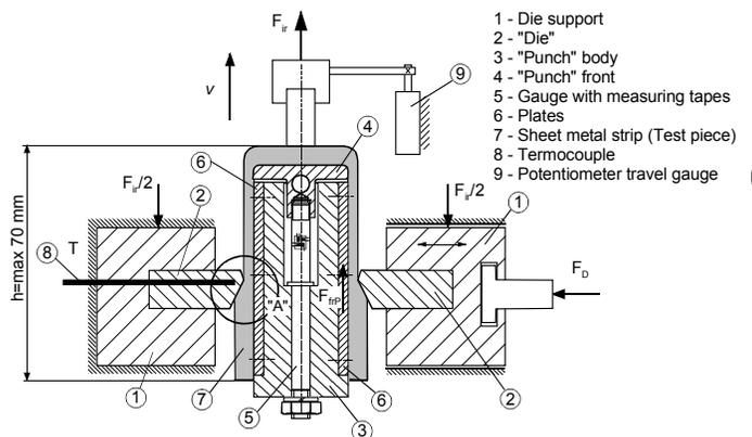
Fig.1 - Scheme of model used in this paper
