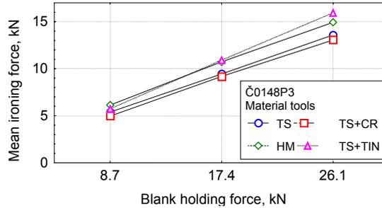
Fig.2. Change of mean value of drawing force in dependence on blank holding force at various tool materials
