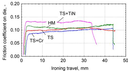
Fig.6 - Friction coefficient for various tool materials
