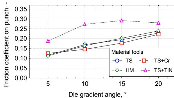
Fig.8 - Change of friction coefficient on punch in dependence on die gradient angle at various tool materials
