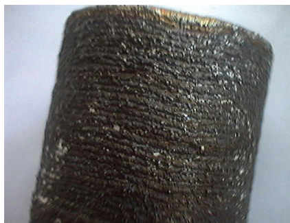
Figure 4 - Structure of side surface of LENS produced specimen
