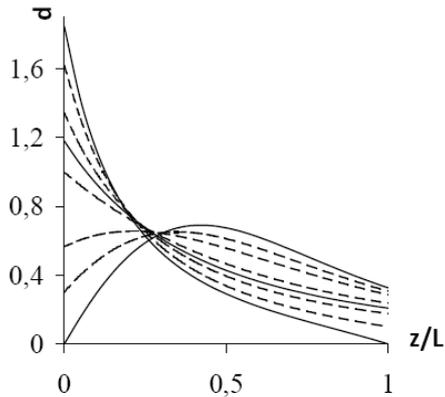
Figure 6 - The sensitivity of the magnitude of the strain rate intensity factor to die geometry
