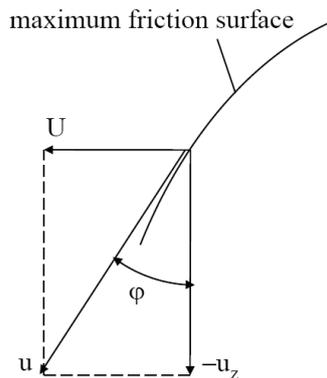
Figure 3 – Components of the velocity vector
