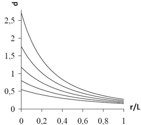
Figure 7 - The sensitivity of the magnitude of the strain rate intensity factor to billet radius
