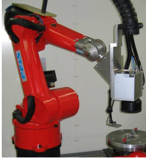
Figure 2 - Remote cutting station holding a high speed scanner
