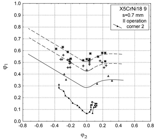
Figure 8 - Strains distribution in LFD for corner 2 in II operation
