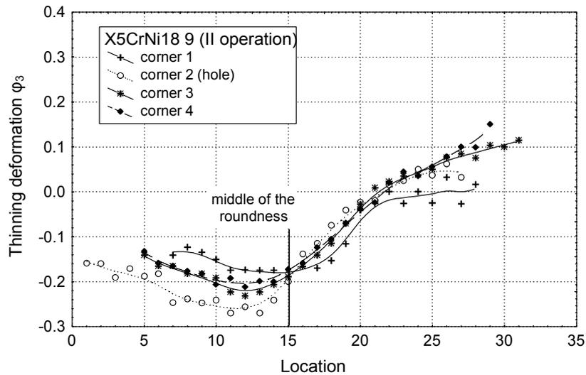
Figure 9 - Thickness strain distribution in II operation
