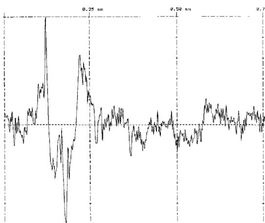
Figure 1 - Surface roughness in the rolling direction
