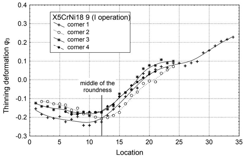
Figure 7 - Thickness strain distribution in I operation
