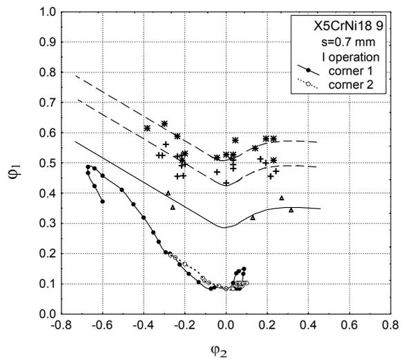
Figure 5 - Limit formability diagram with strain distributions
