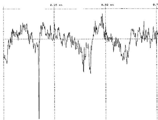
Figure 2 - Surface roughness in the direction 45° towards rolling direction
