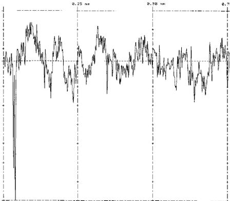
Figure 3 - Surface roughness (direction  $90^\circ$  towards direction of rolling)
