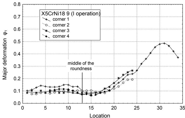
Figure 6 - Larger strain distribution in plane in I operation
