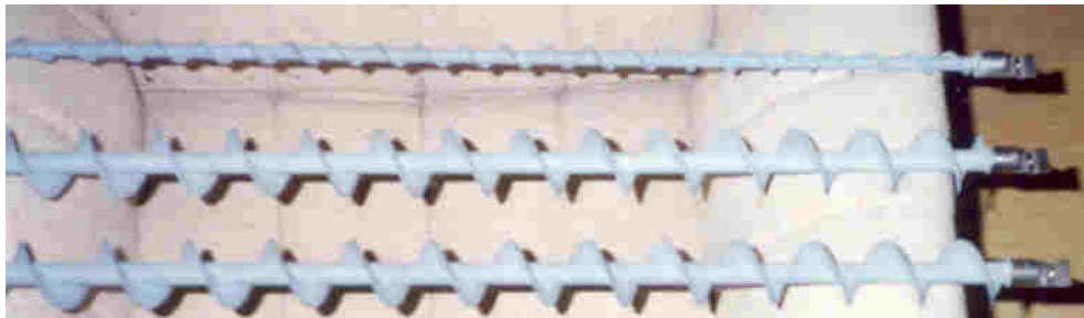
Fig. 3 – Experimentally made samples of spiral conveyors with ceramic coating
