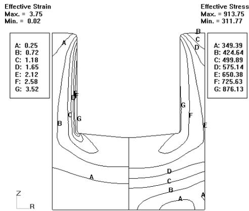
Figure 8. Distribution of effective strain (left) and effective stress (right) ( $s = 10 \text{ mm}$ )
