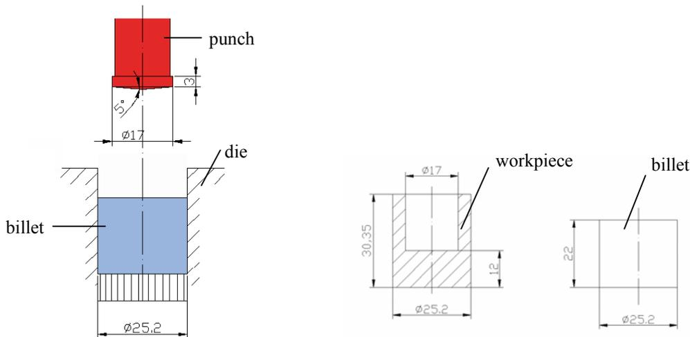
Figure 2. Backward extrusion process, workpiece and billet dimensions
