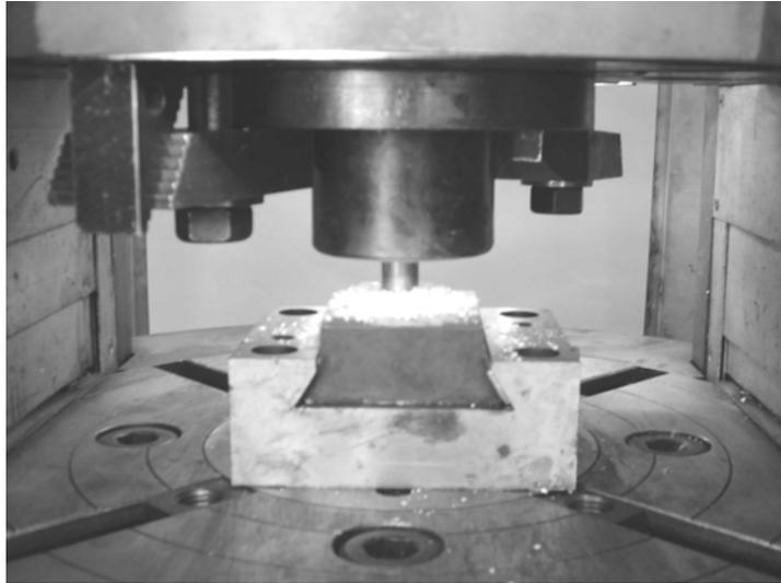
Figure 12. Cylinder strewed with stearin ready for compression
