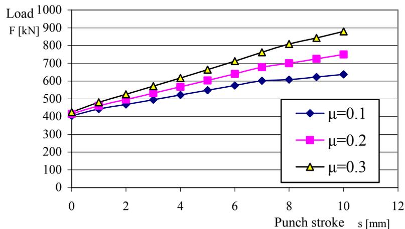
Figure 4. Influence of friction on deformation force
