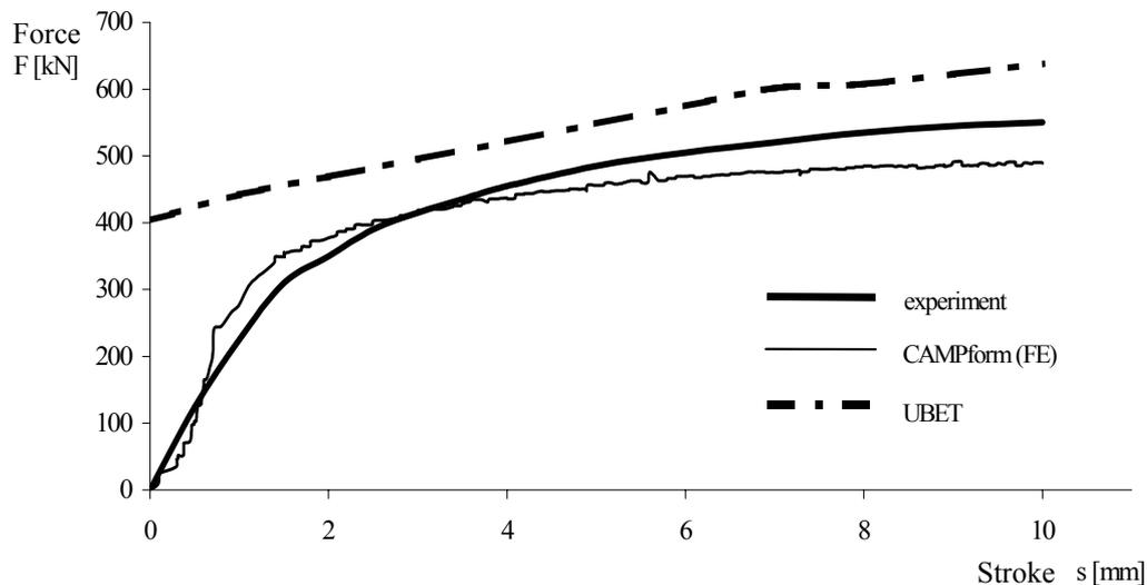
Figure 17. Force – stroke diagram obtained by different methods
