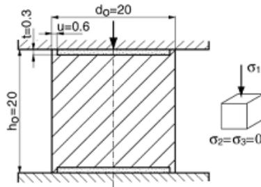
Figure 11. Billet geometry for Rastegaiev method
