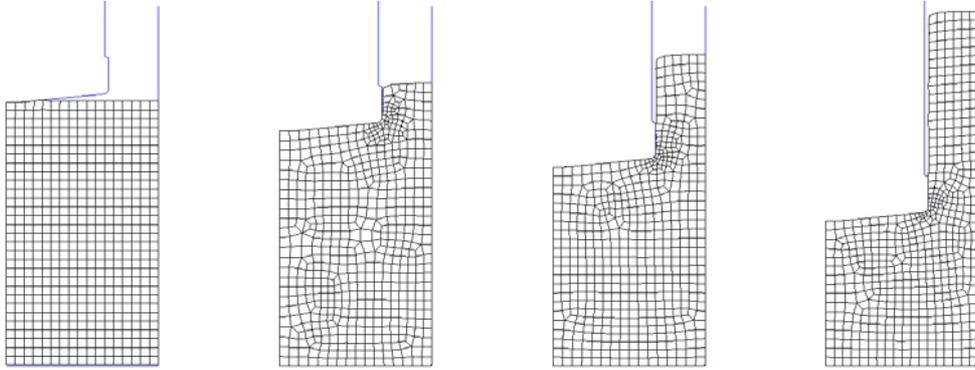
Fig. 10. Alteration of FE mesh in one half of workpiece during deformation process (in 4 steps)
