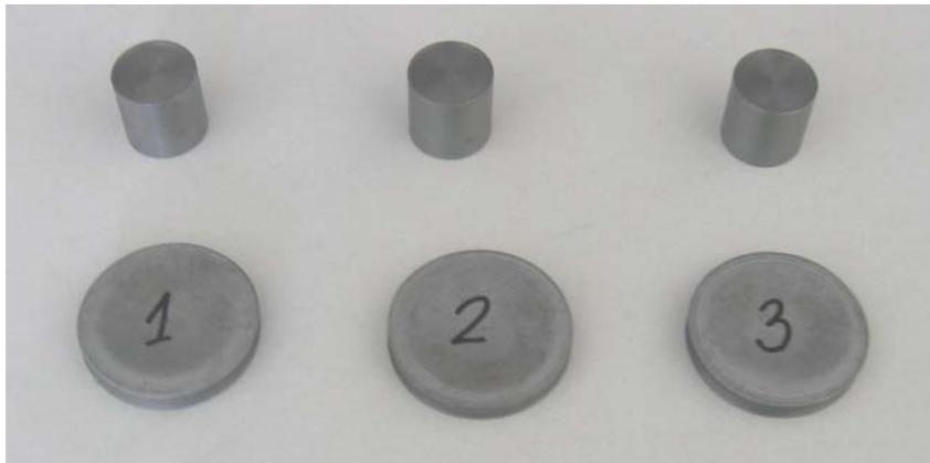
Figure 13. Cylinders before and after compression in Rastegaiev test
