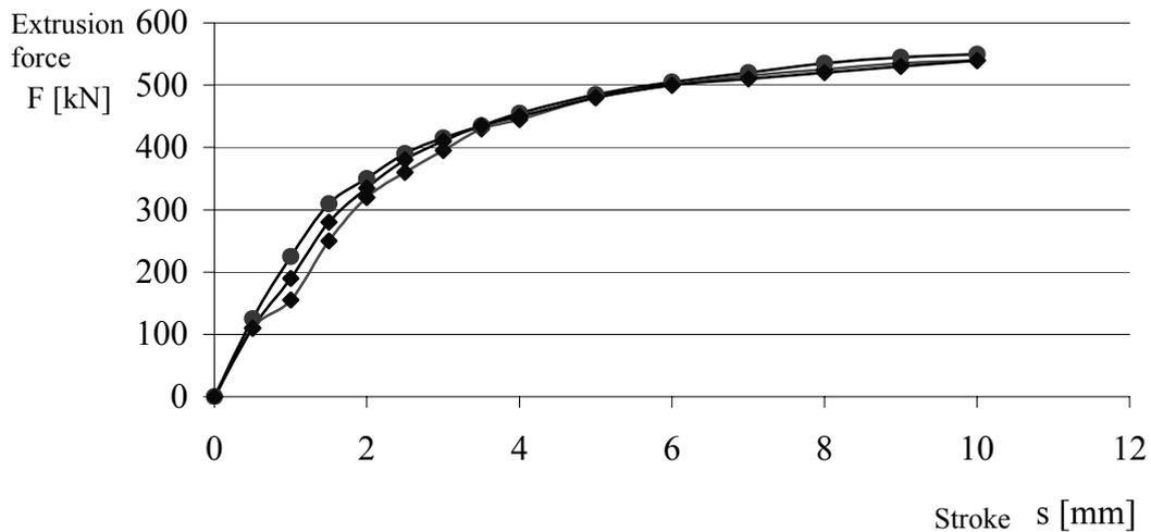
Figure 15. Force – stroke diagram for three specimens
