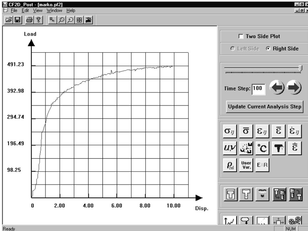
Figure 9. Force – stroke diagram obtained by FE
