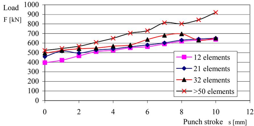
Figure 5. Dependence between force and number of generalized elements
