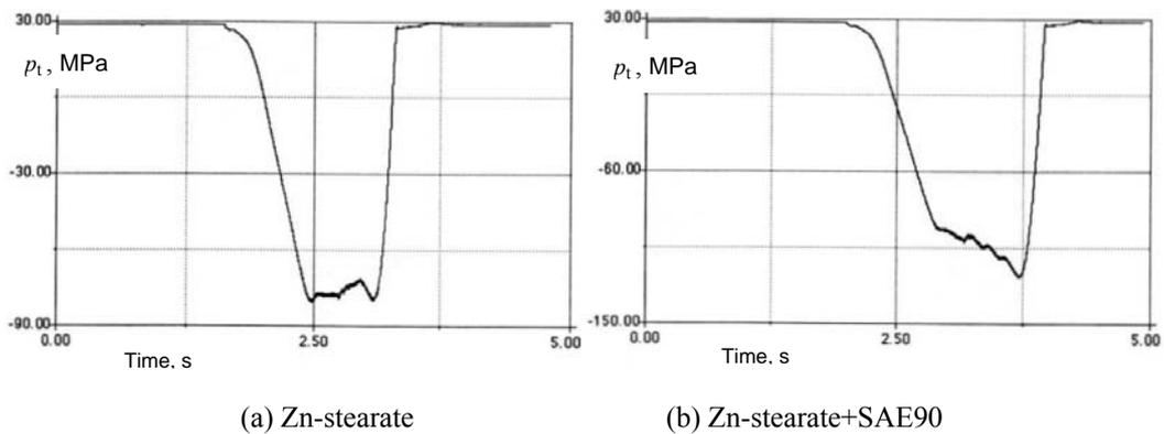
Fig. 5. The pressure-time diagrams for the extrusion with conical punch and  $\varepsilon = 89\%$ .
