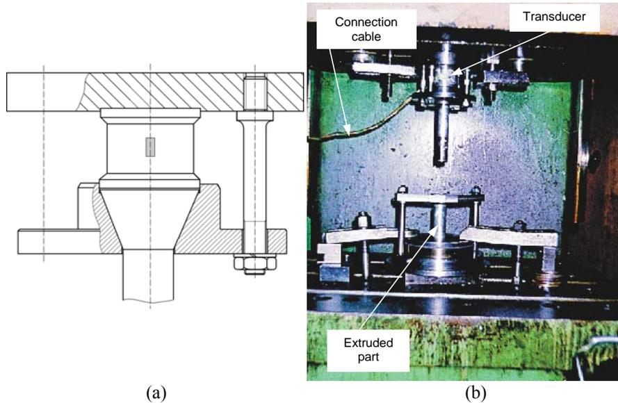
Fig. 2. The detail of extrusion tool with transducer (a) and the tool in working position (b).
