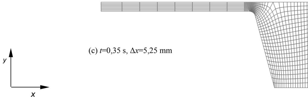
Fig. 7. The numerical grids for simulation of extrusion with conical punch in different time steps: (a) the initial grid,  $t = 0$  s,  $\Delta x = 0$ , (b) the rigid-plastic zones distribution in  $t = 0,35$  s, and  $\Delta x = 1,5$  mm, (c) the final grid after  $t = 0,35$  s and  $\Delta x = 5,25$  mm.
