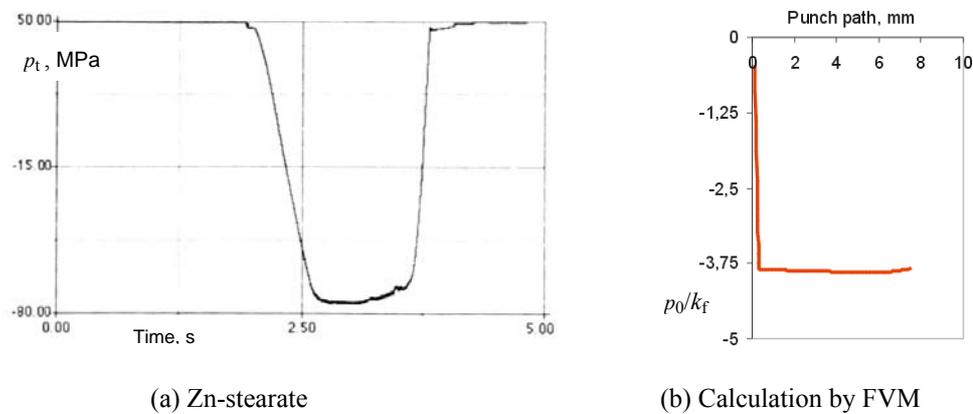
Fig. 4. The pressure – time diagram (a) and the  $p_0/k_f$  – punch path diagram (b), for the extrusion with flat punch and  $\varepsilon = 89\%$ .
