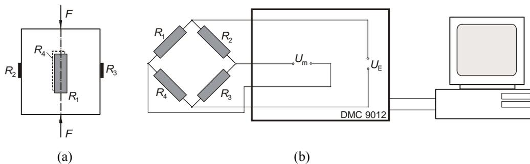
Fig. 1. The scheme of transducer (a), and measuring principle (b).
