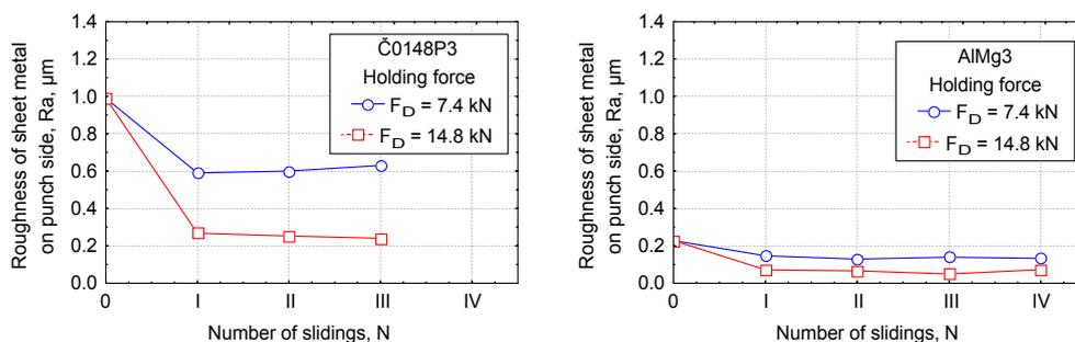
Figure 16 The influence of holding force per drawing phases onto the sheet metal roughness on punch side
