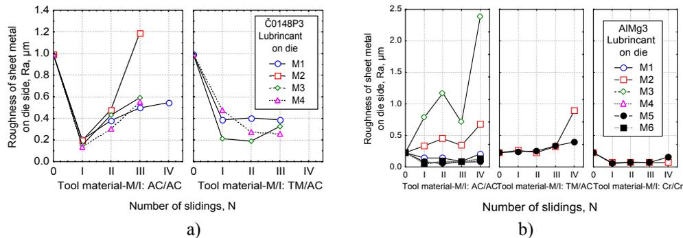
Figure 14 The influence of lubricant onto the sheet metal roughness on die side at different tool materials per drawing phases
