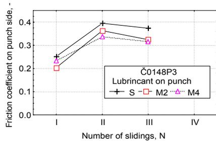
Figure 10 The influence of lubricant on punch per drawing phases onto the friction coefficient  $\mu_I$
