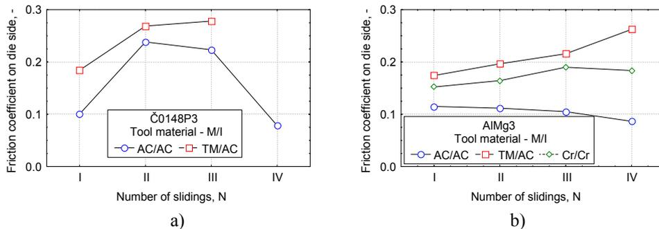
Figure 8 The influence of tool material onto the friction coefficient on die per drawing phases
