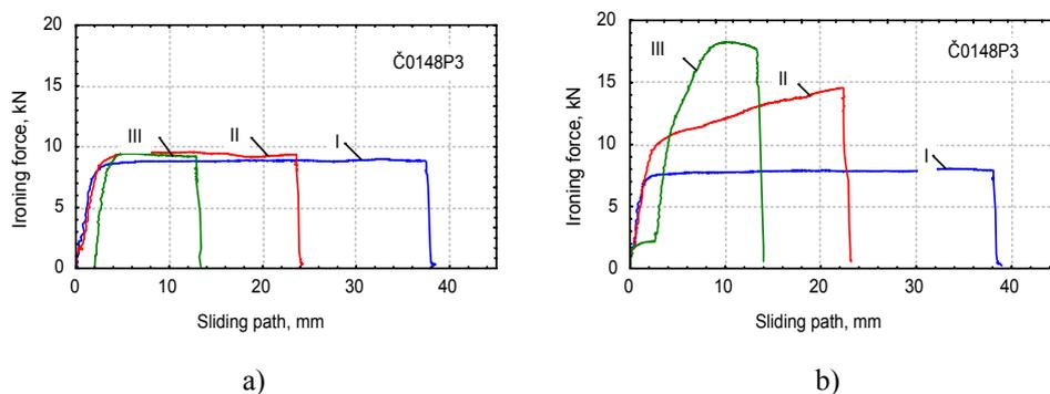
**Figure 4** Change of ironing force at multiphase drawing of steel sheet metal samples
