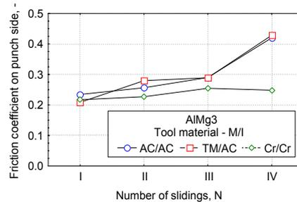
Figure 11 The influence of tool material on punch per drawing phases onto the friction coefficient  $\mu_I$
