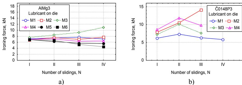
Figure 7 The influence of lubricant on die onto the ironing force per drawing phases
