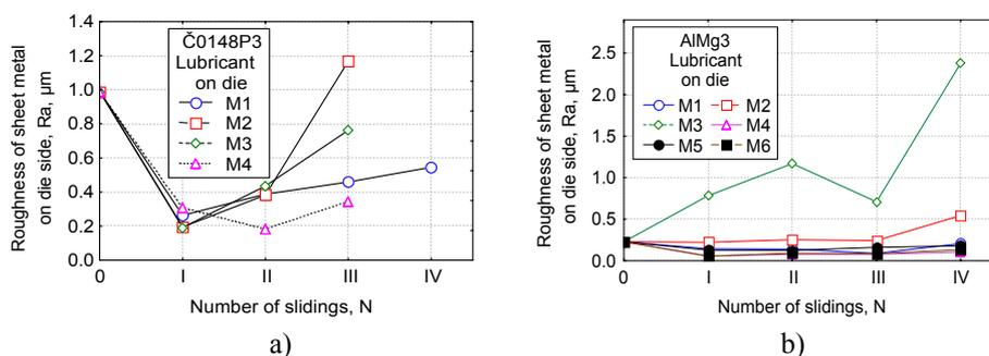
Figure 12 The influence of lubricant onto the die side per drawing phases
