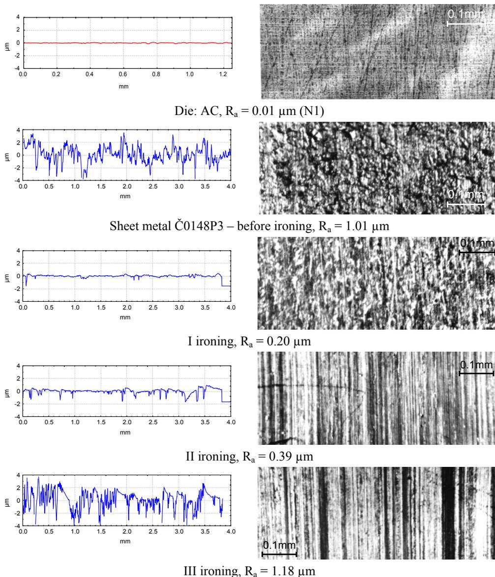
Figure 13 2D roughness form and microphotographs of steel sheet metal surfaces on die side, made at different drawing phases (lubricant on die/punch- M2/S)
