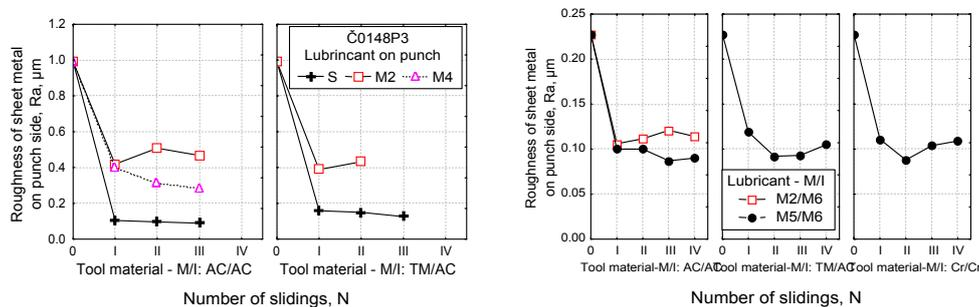
Figure 15 The influence of lubricant on punch onto the sheet metal roughness on punch side at different tool materials per drawing phases
