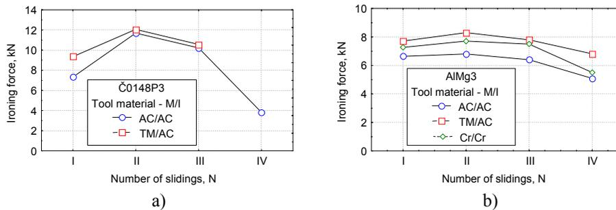
Figure 6 Influence of tool material onto the ironing force per drawing phases
