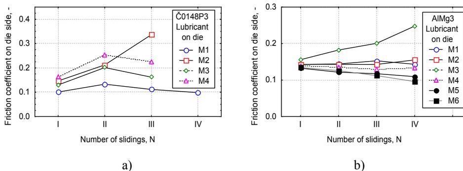
Figure 9 The influence of lubricant on die onto the friction coefficient on die per drawing phases
