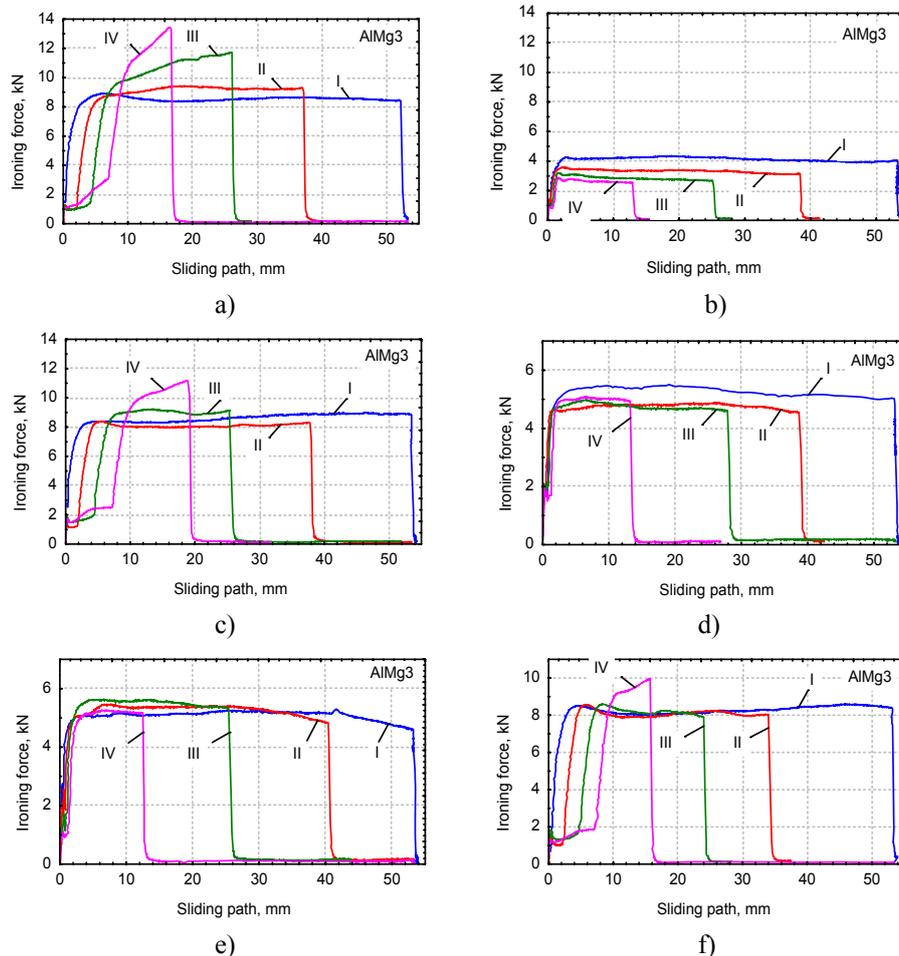
Figure 5 Change of ironing force at multiphase drawing of AlMg3 alloy samples
