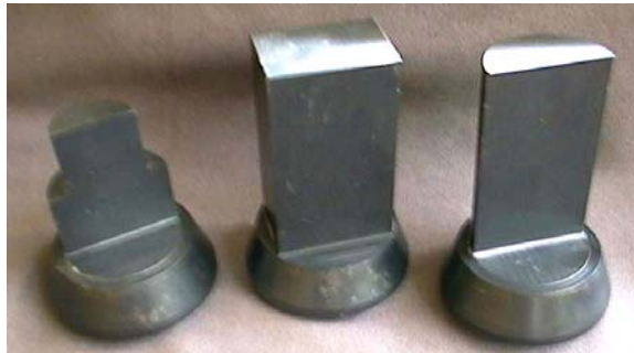
Figure 8 – Punches for backward, plane-strain and forward extrusion
