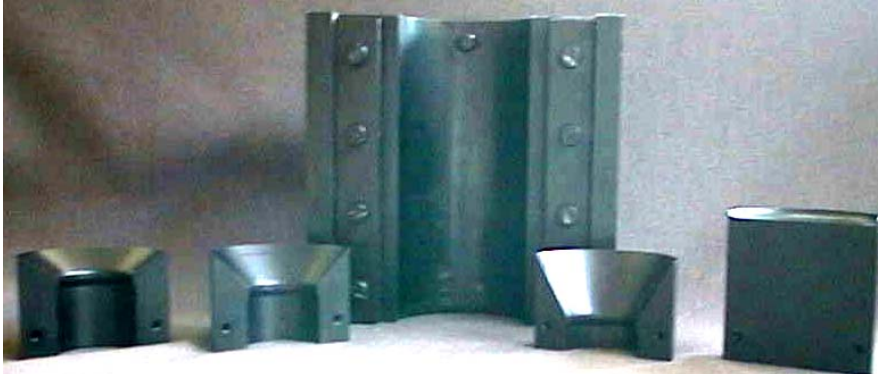
Figure 7 – Die and inserts, for axis-symmetrical extrusion of semi-cylindrical prepared parts
