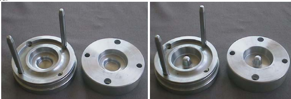
Figure 9 – Tools for modelling of the process of axis-symmetrical forging
