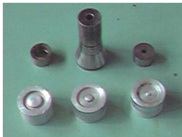
Fig.4. Punch, punch inserts and workpieces
