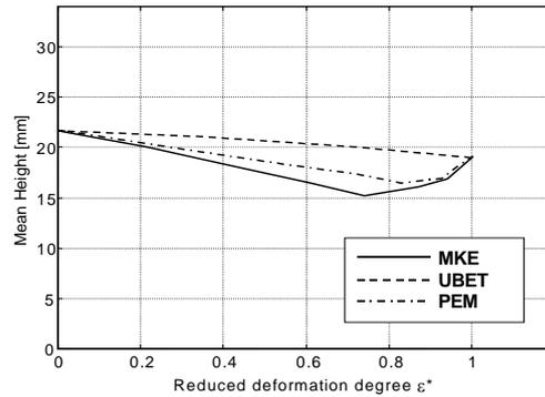
*Fig.13 Mean height of the front contour in the function of a reduced deformation degree*
