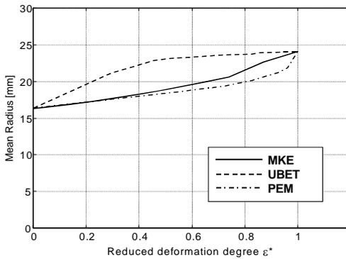
*Fig.12 Mean radius of the side contour in the function of a reduced deformation degree*
