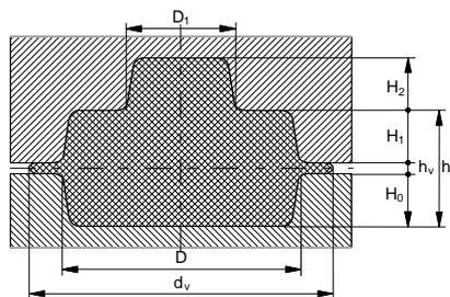
Fig.2. Workingpiece in seizure with die in final phase
