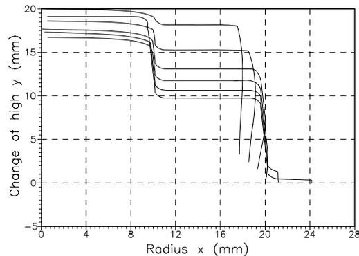
Fig.9 Change in upper workingpiece contour
