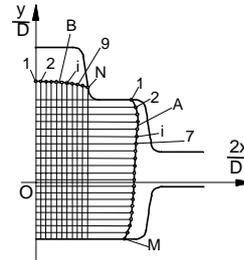
Fig.5 Free workingpiece contour. A - side; B - head
