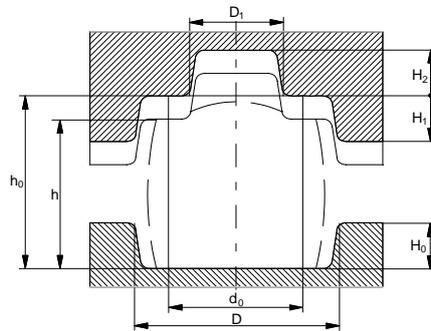
Fig.3 Working piece seized with die in the course of deformation
