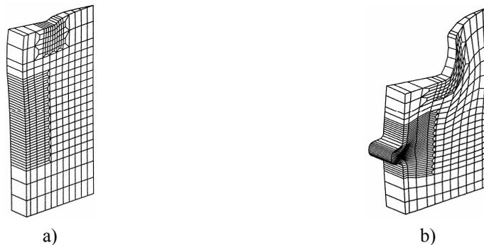
Fig.6 Spacious view of divided body: a) on the began deformation, b) after high deformation
