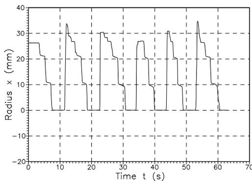
Fig.8 Signal from the inductance sensor in radial direction
