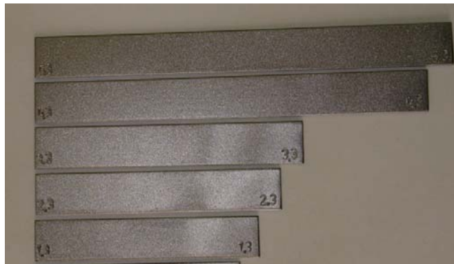
Fig. 1 - Selected samples before bending
