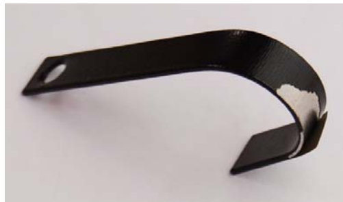
Fig. 8 - Photo without application of plasma - coating BLACK BIG TRUCK
