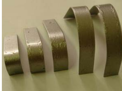
Fig. 5 - Photo of damaged coating STEEL after the bending without application of plasma
