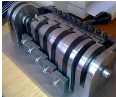
Fig. 10 - Photo of graduated bending jig with rollers with specimens without application of plasma (coating BLACK BIG TRUCK)
