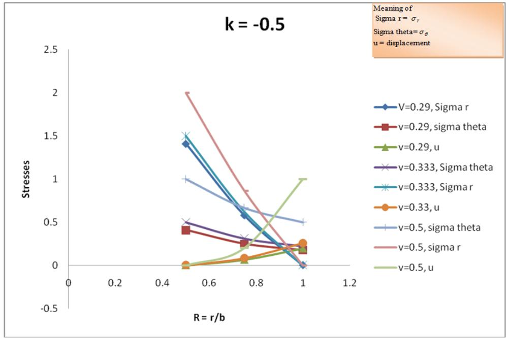
Fig. 3a - Stresses and Displacement at the elastic-plastic Transition state.
