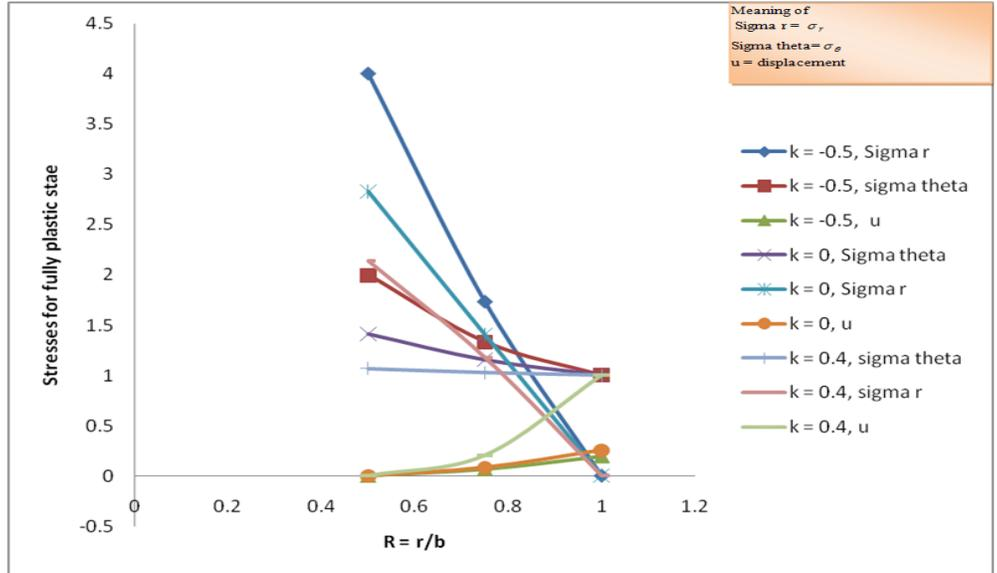
Fig. 4 - Stresses and displacement for fully plastic state
