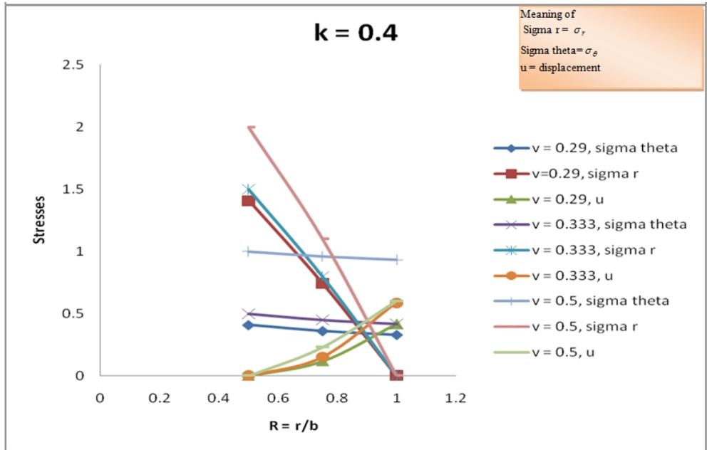
Fig. 3b (2) - Stresses and Displacement at the elastic-plastic Transition state
