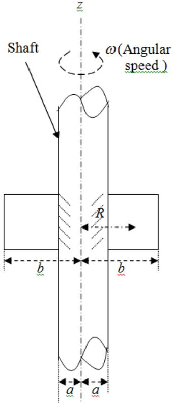
Fig. 1 - Geometry of Rotating Disc.
