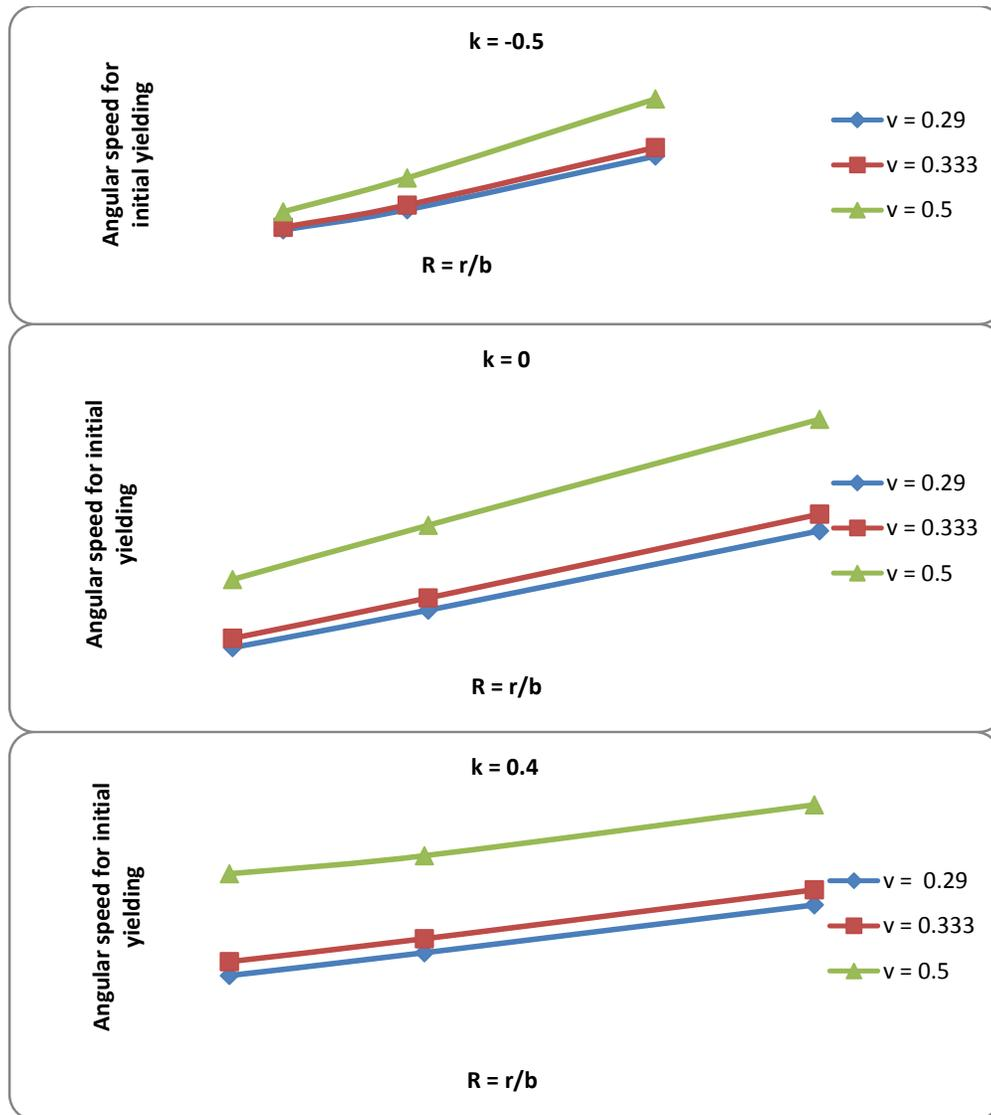
*Fig. 2 - Angular speed required for initial yielding at the internal surface of the rotating disc with rigid inclusion having variable thickness  $k = -0.5, 0, 0.4$  along the radii ratio  $R_0 = a/b$*
