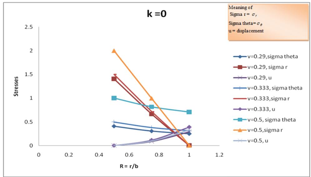
Fig. 3b (1) - Stresses and Displacement at the elastic-plastic Transition state
