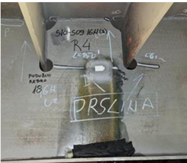
Fig. 6 The cracks propagation ( L_1=150 mm and L_2=80 mm) from the edges of the opening formed during the manufacturing process
