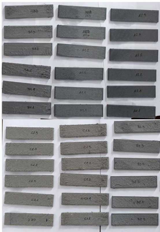
Fig. 5 The appearance of the specimens after 3D printing and cleaning with Sika Cleaner P.
