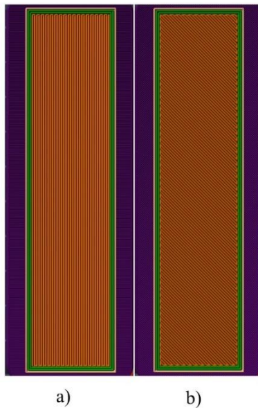
Fig. 3 a) Fiber orientation in the direction of the longitudinal axis of the specimen; b) fiber orientation at an angle of 45° in relation to the longitudinal axis of the specimen.
