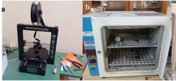
Fig. 2 presentations of (a) Wanhao Duplicator i3 Plus 3D printer; (b) industrial-grade oven
