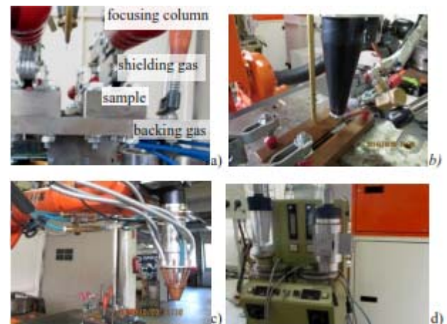
Fig. 1 Installation for this work a) arrangement of the experiment b) wire position in front of laser beam c) head of powder additoner concentric with laser power column d) Sultzer Metco powder self-feeding
