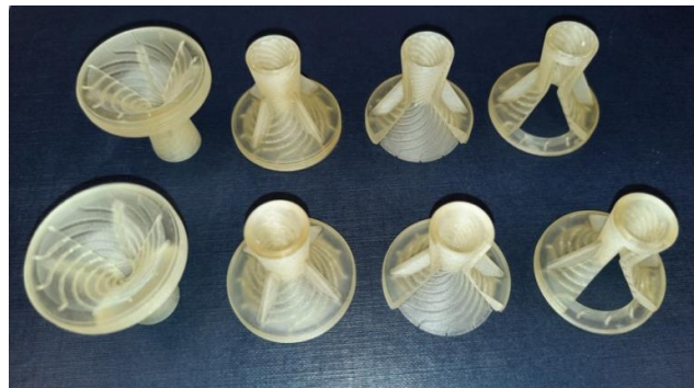
Fig. 12 Fabricated nozzle demonstrators after support material removal
